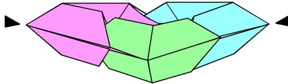
10. Add the third module to the assembly at the front like this. Gently nudge the corners of each module inwards until they fit firmly together.
