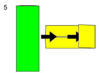
5. Insert a second partly folded module underneath the front flap to act as a template.
